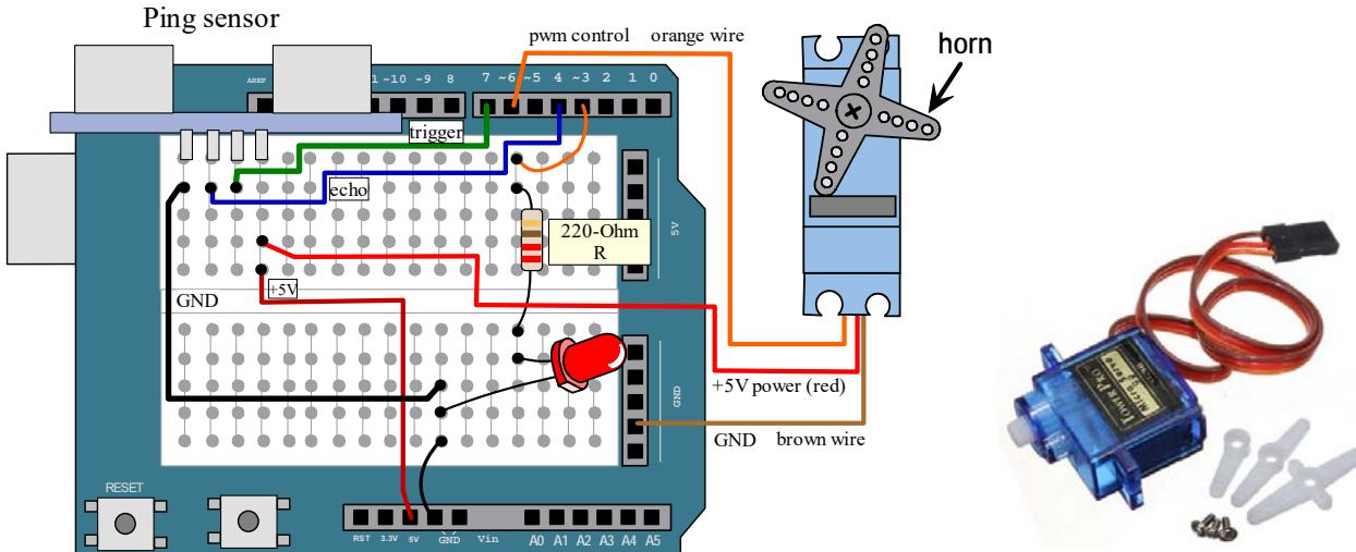
In a prior lab we have learned to control the lighting of an LED, and we have learned to collect distance data from a ultrasonic "ping" sensor. Now we'll learn to control the movement of a servo motor. After that we'll put things together by using the ping distance data to control the LED and the servo.
