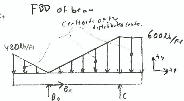
We can replace the distributed forces with concentrated forces at the centroids of the loads
