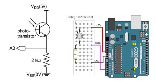
Connect the components as shown. A3 is an analog input on Arduino. Arduino analog inputs use 10-bit analog-to-digital conversion over a range of 0 - 5 V. This means they break up the voltage (range: 0 - 5 V) into 1024 ( $2^{10}$ ) levels. Vdd is 5 VDC. While the phototransistor controls how much current flows, the resistor is needed to transform current into a readable voltage. The resistor should be at least  $2k\Omega$  to restrict current draw on the Arduino to just a couple of mA.
