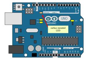
Here we get the "surface mounted" (built onto the board) LED (connected to pin 13) to blink on and off.
